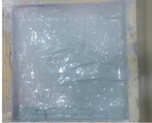
Figure 1. illustrates the composite material composed of epoxy resin reinforced with reed fibers
