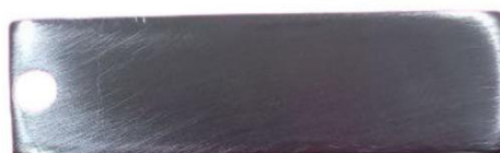
Figure 2. Shape of the N-80 carbon steel oil pipe samples used
